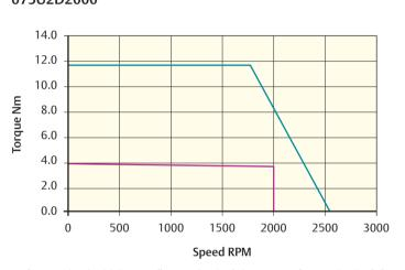
Peak torque (Nm) = 6.6 Stall torque (Nm) = 2.2 Rated torque (Nm) = 2.1 Peak torque (Nm) = 11.7 Stall torque (Nm) = 3.9 Rated torque (Nm) = 3.8
