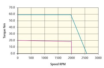
Stall torque (Nm) = 19.8 Peak torque (Nm) = 59.4 Rated torque (Nm) = 18.4
