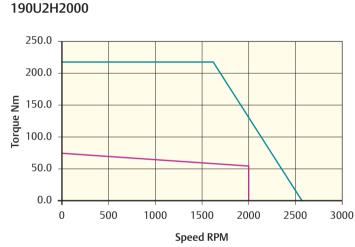
Peak torque (Nm) = 219.6 Stall torque (Nm) = 73.2 Rated torque (Nm) = 54.7
