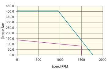
Peak torque (Nm) = 408.0 Stall torque (Nm) = 136.0 Rated torque (Nm) = 84.0
