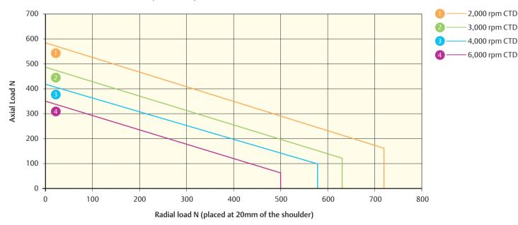
$75U2L_{10(h)}$  Bearing life for 20,000 hours (reliability 90%, load factor of 1). Do not exceed a maximum axial load of 900 N
