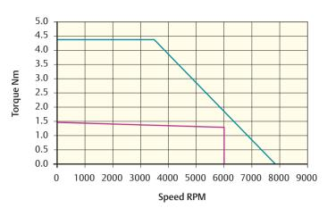
Stall torque (Nm) = 1.45 Rated torque (Nm) = 1.30 Peak torque (Nm) = 4.35
