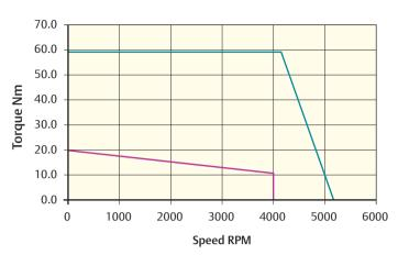
Peak torque (Nm) = 59.4 Stall torque (Nm) = 19.8 Rated torque (Nm) = 10.7
