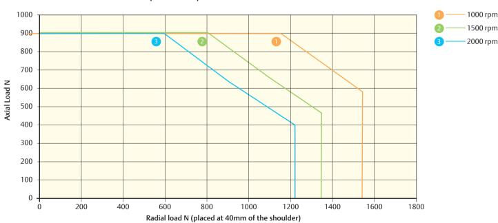
$190 \text{UD L}_{_{10(\text{h})}} \text{Bearing life for 20,000 hours (reliability 90\%, load factor of 1)}. Do not exceed a maximum axial load of 900 \, \text{N}$
