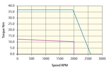
Peak torque (Nm) = 37.2 Stall torque (Nm) = 12.4 Rated torque (Nm) = 10.8
