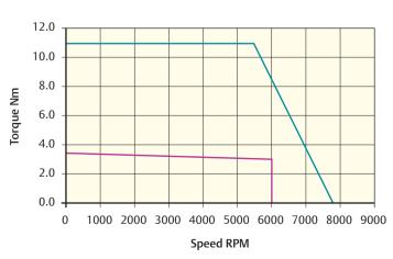
Peak torque (Nm) = 11.10 Stall torque (Nm) = 3.70 Rated torque (Nm) = 3.10
