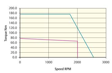
Peak torque (Nm) = 176.10 Stall torque (Nm) = 79.0 Rated torque (Nm) = 66.5
