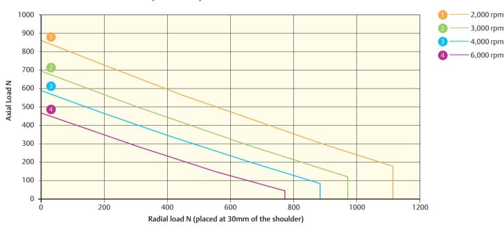
$115 \text{UD L}_{_{10(h)}} \text{Bearing life for 20,000 hours (reliability 90\%, load factor of 1)}. Do not exceed a maximum axial load of 1200 \, N \\$
