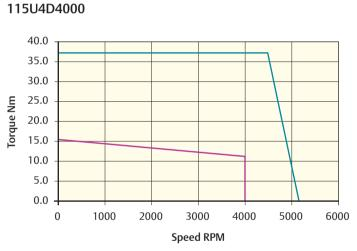
Peak torque (Nm) = 37.20 Stall torque (Nm) = 15.2 Rated torque (Nm) = 12.0
