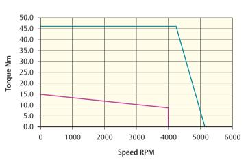
Peak torque (Nm) = 45.9 Stall torque (Nm) = 15.3 Rated torque (Nm) = 8.7
