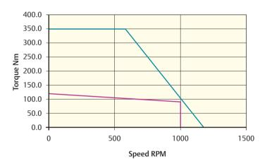
Peak torque (Nm) = 348.0 Stall torque (Nm) = 116.0 Rated torque (Nm) = 92.0
