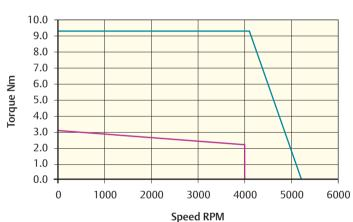
Peak torque (Nm) = 9.3 Stall torque (Nm) = 3.1 Rated torque (Nm) = 2.3
