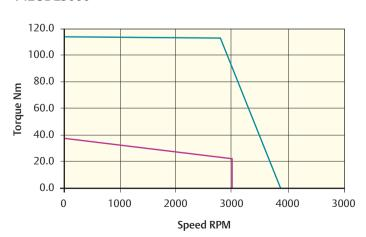
$Peak torque (Nm) = 114.00 \quad Stall torque (Nm) = 38.00 \quad Rated torque (Nm) = 23.00$
