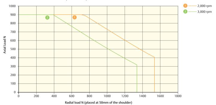
$190U2\ L_{10(h)}$  Bearing life for 20,000 hours (reliability 90%, load factor of 1). Do not exceed a maximum axial load of 900 N
