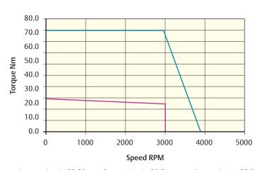
Peak torque (Nm) = 70.20 Stall torque (Nm) = 29.5 Rated torque (Nm) = 25.0
