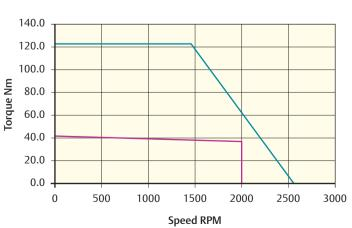
Peak torque (Nm) = 123.3 Stall torque (Nm) = 41.1 Rated torque (Nm) = 36.9
