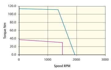
Peak torque (Nm) = 114.00 Stall torque (Nm) = 38.00 Rated torque (Nm) = 31.70
