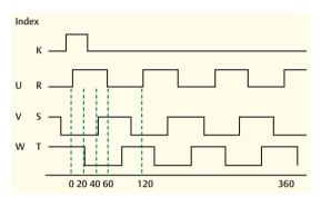
Where N = number of poles. For example a 6 pole motor the encoder commutation tracks will output 3 pulses per channel per revolution and for an 8 pole motor the encoder commutation tracks will give 4 pulses per channel per revolution.
