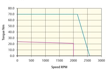
Peak torque (Nm) = 70.4 Stall torque (Nm) = 23.4 Rated torque (Nm) = 21.3
