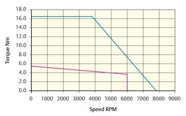
Peak torque (Nm) = 16.50 Stall torque (Nm) = 5.50 Rated torque (Nm) = 3.80
