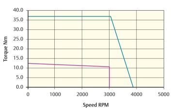
Peak torque (Nm) = 37.4 Stall torque (Nm) = 12.4 Rated torque (Nm) = 10.4
