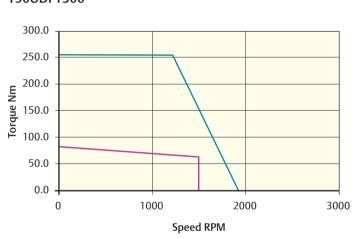
$\text{Rated torque (Nm) = 42.50} \qquad \text{Peak torque (Nm) = 255.00} \qquad \text{Stall torque (Nm) = 85.00} \qquad \text{Rated torque (Nm) = 68.50}$
