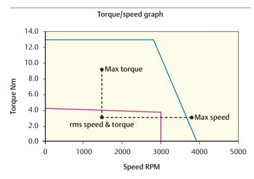
Max torque = 10Nm: Max speed = 3900 rms torque = 3Nm: rms speed = 1500
