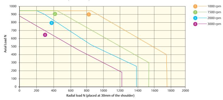
$142 UD\ L_{_{10(h)}}\ Bearing\ life\ for\ 20,000\ hours\ (reliability\ 90\%,\ load\ factor\ of\ 1).\ Do\ not\ exceed\ a\ maximum\ axial\ load\ of\ 950\ N$
