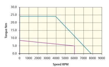
Peak torque (Nm) = 24.00 Stall torque (Nm) = 8.00 Rated torque (Nm) = 5.00
