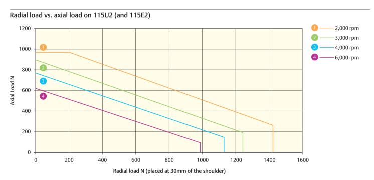
$115 U2\ L_{_{10(h)}} Bearing\ life\ for\ 20,000\ hours\ (reliability\ 90\%,\ load\ factor\ of\ 1).\ Do\ not\ exceed\ a\ maximum\ axial\ load\ of\ 950\ N$
