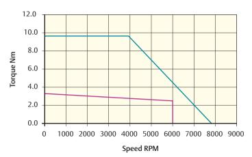
Peak torque (Nm) = 9.60 Stall torque (Nm) = 3.20 Rated torque (Nm) = 2.65
