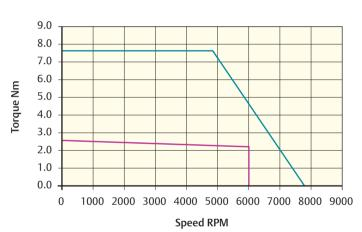
Peak torque (Nm) = 7.65 Stall torque (Nm) = 2.55 Rated torque (Nm) = 2.20
