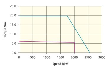
Peak torque (Nm) = 19.8 Stall torque (Nm) = 6.6 Rated torque (Nm) = 6.1
