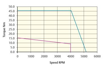
Peak torque (Nm) = 45.9 Stall torque (Nm) = 15.3 Rated torque (Nm) = 8.9
