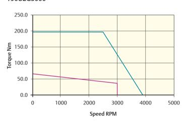
Peak torque (Nm) = 123.3 Stall torque (Nm) = 41.1 Rated torque (Nm) = 33.0
