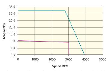
Peak torque (Nm) = 32.4 Stall torque (Nm) = 10.8 Rated torque (Nm) = 9.0
