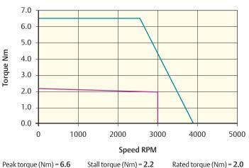
Stall torque (Nm) = 2.2 Rated torque (Nm) = 2.0
