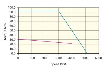
Peak torque (Nm) = 93.3 Stall torque (Nm) = 31.1 Rated torque (Nm) = 21.5
