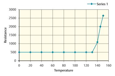
The installer must connect the motor thermistor to the drive to cause motor power shutdown in the event of overheating. It is the installer's responsibility to ensure that this protection facility is properly connected and set at the drive.
