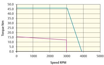
Peak torque (Nm) = 45.9 Stall torque (Nm) = 15.3 Rated torque (Nm) = 12.6
