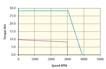
Peak torque (Nm) = 28.2 Stall torque (Nm) = 9.4 Rated torque (Nm) = 8.1
