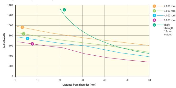
089UD L  $_{_{10(h)}}\mbox{Bearing}$  life for 20,000 hours (reliability 90%, load factor of 1).
