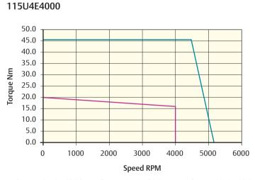
Peak torque (Nm) = 45.90 Stall torque (Nm) = 20.1 Rated torque (Nm) = 16.1
