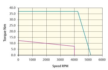
Peak torque (Nm) = 37.2 Stall torque (Nm) = 12.4 Rated torque (Nm) = 7.5
