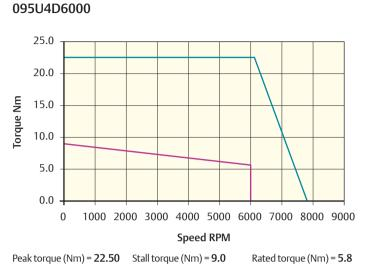
Peak torque (Nm) = 22.50 Stall torque (Nm) = 9.0
