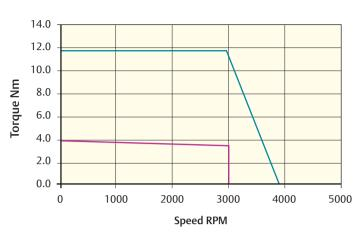
Peak torque (Nm) = 11.7 Stall torque (Nm) = 3.9 Rated torque (Nm) = 3.5
