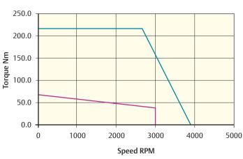
Peak torque (Nm) = 219.6 Stall torque (Nm) = 73.2 Rated torque (Nm) = 36.8
