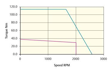
Peak torque (Nm) = 114.00 Stall torque (Nm) = 38.00 Rated torque (Nm) = 29.60
