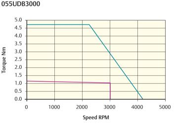
Peak torque (Nm) = **4.72** Stall torque (Nm) = **1.18** Rated torque (Nm) = **1.05**
