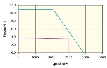
Peak torque (Nm) = 11.10 Stall torque (Nm) = 3.70 Rated torque (Nm) = 3.50
