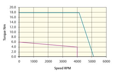
Peak torque (Nm) = 17.7 Stall torque (Nm) = 5.9 Rated torque (Nm) = 4.0
