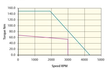
Peak torque (Nm) = 151.6 Stall torque (Nm) = 68.0 Rated torque (Nm) = 55.0
