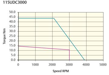
Peak torque (Nm) = 43.80 Stall torque (Nm) = 14.60 Rated torque (Nm) = 10.50
