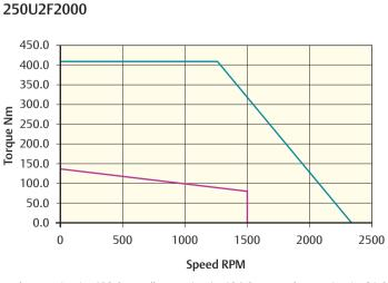
Peak torque (Nm) = 408.0 Stall torque (Nm) = 136.0 Rated torque (Nm) = 81.0
