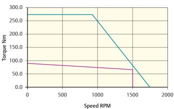
Peak torque (Nm) = 276.0 Stall torque (Nm) = 92.0 Rated torque (Nm) = 67.0
