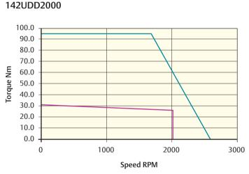
Peak torque (Nm) = 94.50 Stall torque (Nm) = 31.50 Rated torque (Nm) = 25.70
