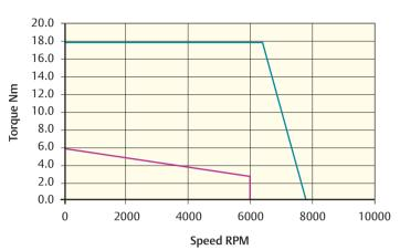
Peak torque (Nm) = 17.7 Stall torque (Nm) = 5.9 Rated torque (Nm) = 2.8
