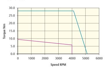
Peak torque (Nm) = 28.2 Stall torque (Nm) = 9.4 Rated torque (Nm) = 6.3
