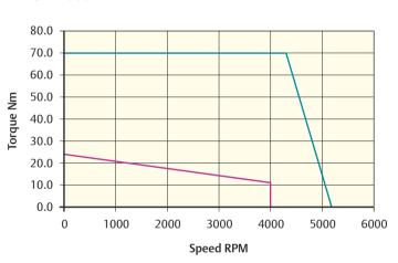
Peak torque (Nm) = 70.2 Stall torque (Nm) = 23.4 Rated torque (Nm) = 12.2
