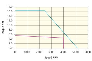
Peak torque (Nm) = 16.50 Stall torque (Nm) = 5.50 Rated torque (Nm) = 4.55
