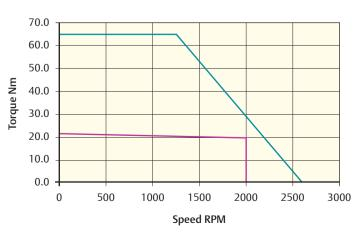
Peak torque (Nm) = 65.4 Stall torque (Nm) = 21.8 Rated torque (Nm) = 20.0
