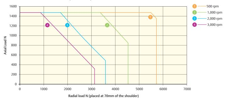
$250U2\,L_{_{10(h)}} Bearing\ life\ for\ 20,000\ hours\ (reliability\ 90\%,\ load\ factor\ of\ 1).\ Do\ not\ exceed\ a\ maximum\ axial\ load\ of\ 1450\ N$
