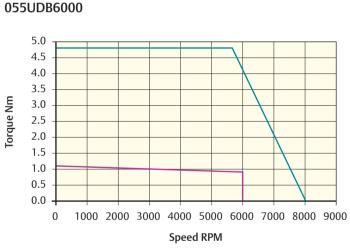
Peak torque (Nm) = 4.72 Stall torque (Nm) = 1.18 Rated torque (Nm) = 0.90
