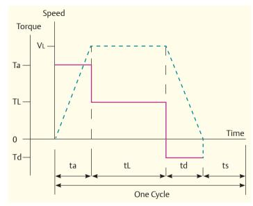
From the above speed-torque diagram calculate the rms torque using the formula:
