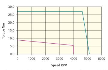
Peak torque (Nm) = 27.0 Stall torque (Nm) = 9.0 Rated torque (Nm) = 5.7
