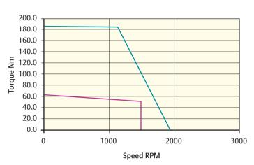
Peak torque (Nm) = 186.00 Stall torque (Nm) = 62.00 Rated torque (Nm) = 52.20
