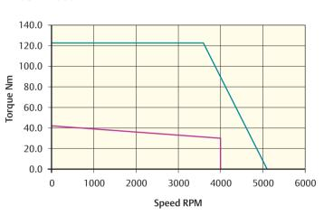
ak torque (Nm) = 65.4 Stall torque (Nm) = 21.8 Rated torque (Nm) = 17.5 Peak torque (Nm) = 123.3 Stall torque (Nm) = 41.1 Rated torque (Nm) = 29.0
