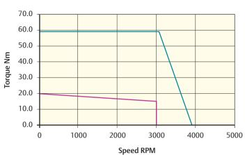
Peak torque (Nm) = 59.4 Stall torque (Nm) = 19.8 Rated torque (Nm) = 15.8
